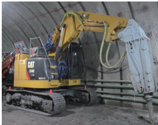
T-PROBO : A model specializing in tunnel construction. Compatible with 8t, 15t and 20t class hydraulic excavators.
