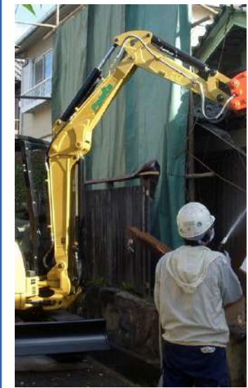
2-position boom exclusively for mini excavators Paletta
