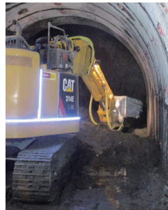
T-PROBO : A model specializing in tunnel construction. Compatible with 8t, 15t and 20t class hydraulic excavators.
