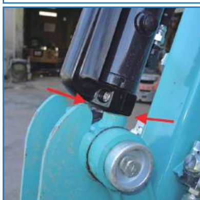
⑤ Make a final check by moving the hydraulic cylinders to make sure there is no interference with any part.
