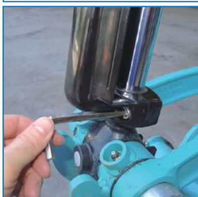
④ Securely tighten the BORG body part and receiving part with screws and nuts.
